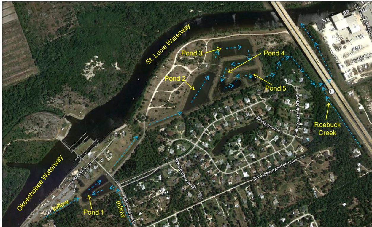
Figure 2-1. Overview of the Tropical Farms Treatment System with Primary Flow Lines.
